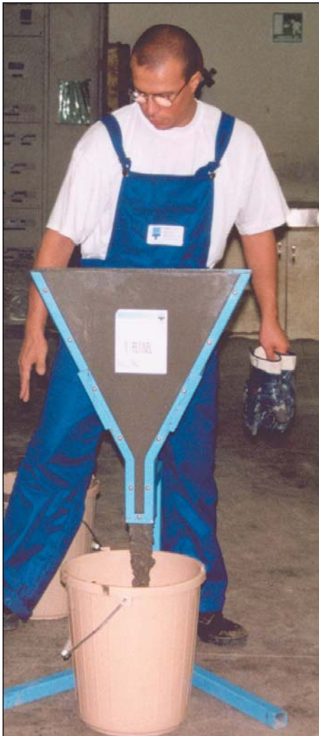
Rheodynamic Concrete Demonstrates Flow Characteristics
