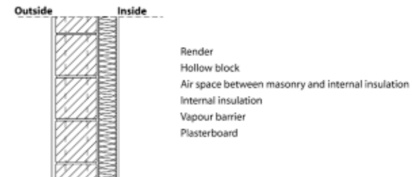
W5 Hollow-block, internal insulation
