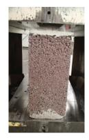
the new test method is substantially equivalent to 5N/mm² under the old test method. Thus, there is really only a change in block strength designation resulting from the changed test method required under I.S. EN 771-3, and manufacturers substantially produce the same block as was previously designated at the lower strength, for all intents and purposes.
