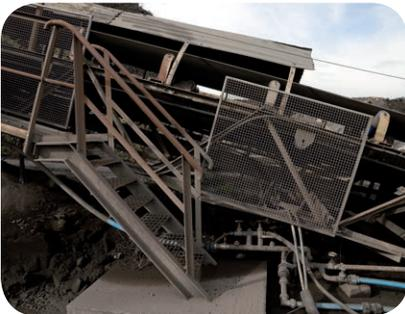
If guarding must be removed for maintenance reasons, then the equipment must be securely isolated and the guarding replaced before the isolation is removed.
