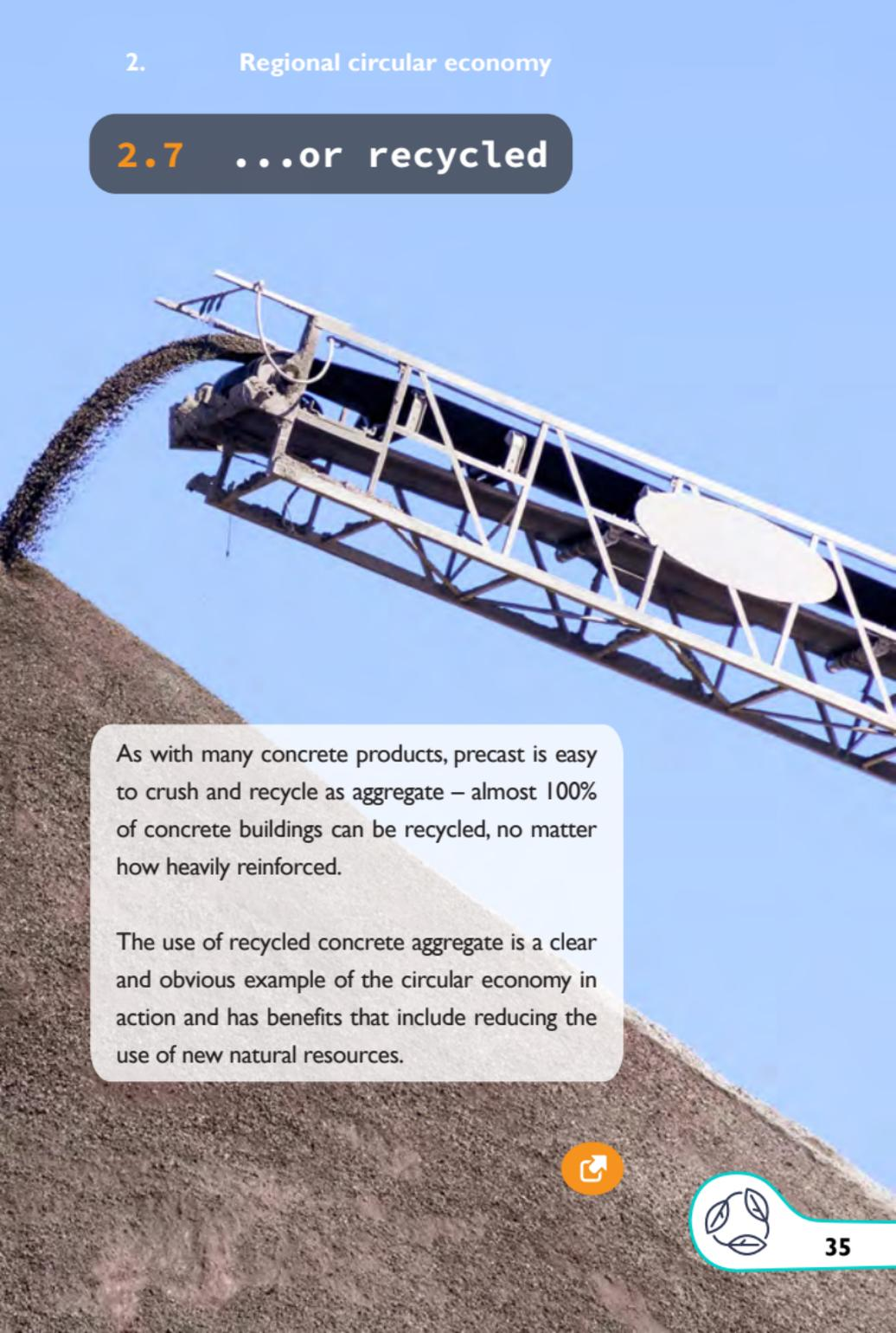
As with many concrete products, precast is easy to crush and recycle as aggregate – almost 100% of concrete buildings can be recycled, no matter how heavily reinforced.
